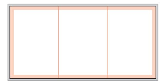
For large custom size boards or signs anything over standard machine sizes will be produced in sections. The diagram above shows a 3000mm x 1500mm with 3 panel splits of 1000mm x 1500mm. If you have special requirements for sizes of the panels please add these to the notes when placing your order and/or uploading files.
