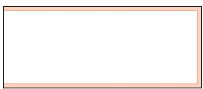
Panel 2 measures 508mm x 1219mm with NO OVERLAP. Panel 2 has safe area on the top, bottom and right hand side. This is 26mm per edge that should contain no text or important image. This is indicated on the diagram in red.
