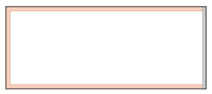
Panel 1 measures 508mm x 1219mm with 12mm of UNPRINTED overlap on the right hand side making it 1231mm at full size. This is indicated on the diagram in grey. The 12mm is at full size please scale accordingly. Panel 1 also has safe area on the top, bottom and left hand side. This is 26mm per edge that should contain no text or important images. This is indicated on the diagram in red.
