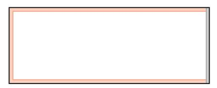
Panel 1 measures 508mm x 1321mm with 12mm of UNPRINTED overlap on the right hand side making it 1333mm at full size. This is indicated on the diagram in grey. The 12mm is at full size please scale accordingly. Panel 1 also has safe area on the top, bottom and left hand side. This is 26mm per edge that should contain no text or important image. This is indicated on the diagram in red.
